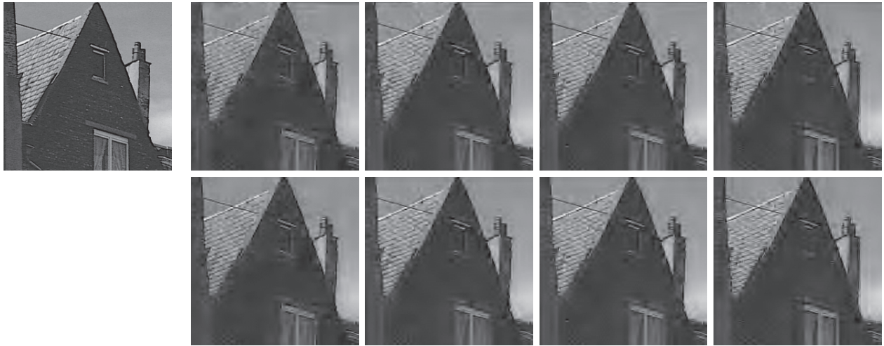
Fig. 6. Comparison of results in a particular area of the image Cafe (top and left sides are boundaries; bitrate: 0.25 [bpp]): (top-left) original image, (other left-to-right) 4 \times 8 HLT, 4 \times 8 ReBLFB, 4 \times 8/4 \times 12 ReBLFB, and 4 \times 12 ReBLFB, (top) a periodic extension, and (bottom) the proposed nonexpansive convolution.
