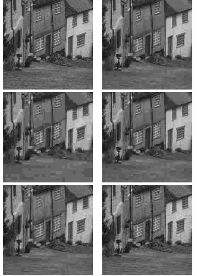
Figure 5: Enlarged images of “Goldhill” for lossy image coding: (top left) original, (top right) using the method of Komatsu et al. [6], (middle left) using the method of Liang et al. [7], (middle right) using the 8-channel proposed method, (bottom left) using the 16-channel proposed method, (bottom right) using the 32-channel proposed method
