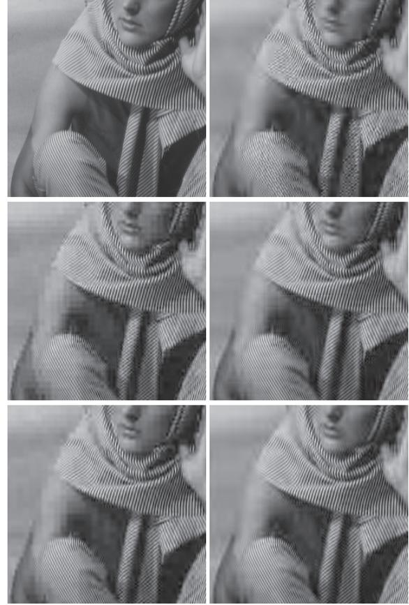
**Fig. 3.** Comparison of a particular area of the reconstructed image *Barbara* (bitrate is 0.25[bpp]): (top) original image and the HLBT for JPEG XR [8], (middle) the conventional  $8 \times 16$  and  $16 \times 32$  FLOTs [10], (bottom) the proposed  $8 \times 16$  and  $16 \times 32$  FLBTs.
