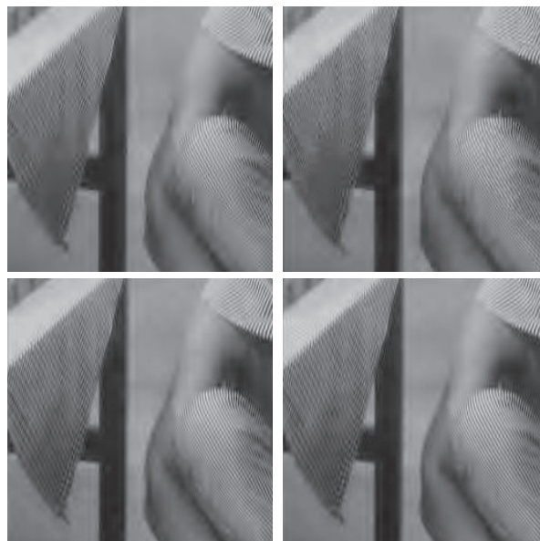
Fig. 6. Comparison of the part of the enlarged images of Barbara (bitrate: 0.25[bpp]): (top-left) 9/7-tap DWT (JPEG2000), (top-right) 4 × 8 HLBT (JPEG XR), (bottom-left) 8 × 24 BOFB ( N = 2 ), (bottom-right) 8 × 24 BOFB ( N = 4 ).
