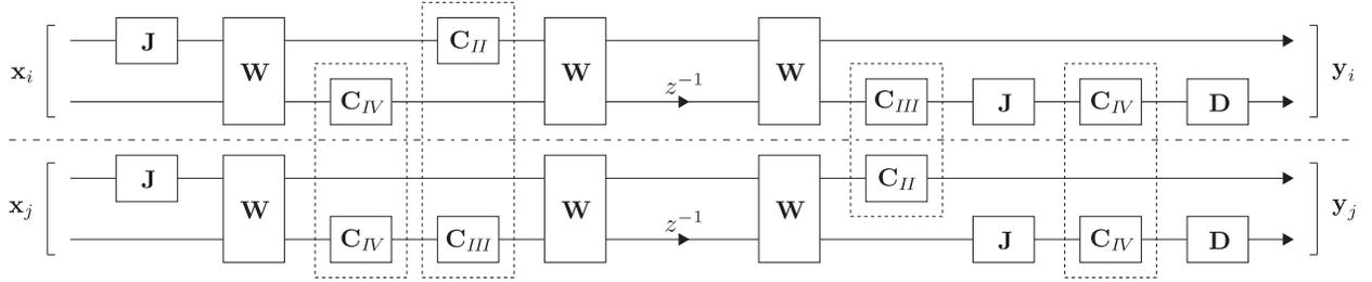
Fig. 2. The parallel process of two different type FLOTs: (top) FLOT in (2), (bottom) FLOT in (3).
