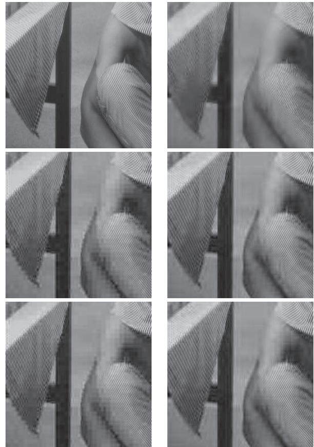
**Fig. 4.** Enlarged images of *Barbara* in lossy image coding (bitrate: 0.25 [bpp]): (top-left) original image, (top-right) HLBT in JPEG XR, (middle-left) conv.  $8 \times 16$  FLOT, (middle-right) conv.  $16 \times 32$  FLOT, (bottom-left) prop.  $8 \times 16$  FLOT, (bottom-right) prop.  $16 \times 32$  FLOT.
