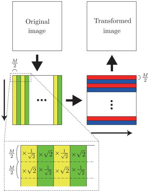
Fig. 3. The process of the two-dimensional transform of an image by the proposed FLOTs.
