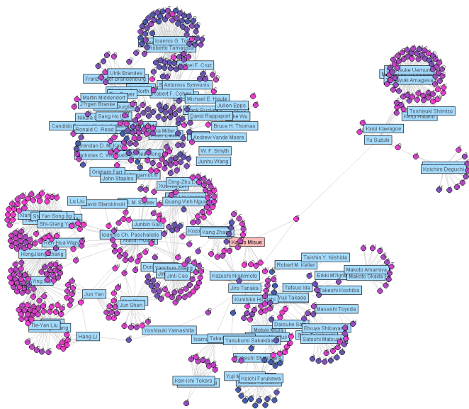
Fig. 1. Examples of a papers/authors network drawn using spring embedder model. Network consists of 117 author nodes (rectangles), 627 paper nodes (small circles), and 1500 edges.
