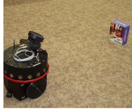
Fig. 8 Experimental environment. The obstacle exists in front of the mobile robot. The mobile robot moves toward the obstacle.
