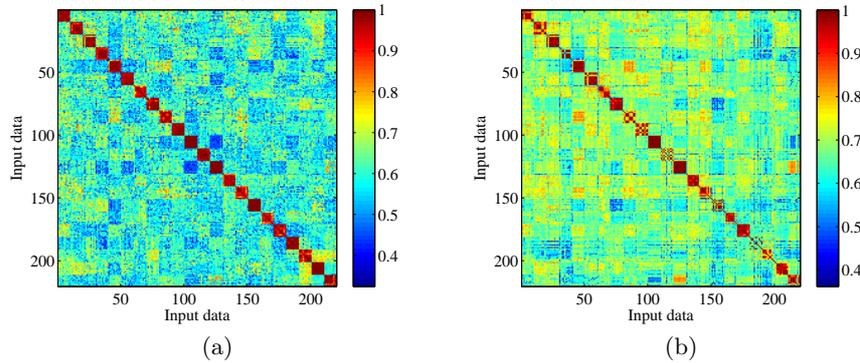
**Fig. 10.** Similarity maps based on the canonical angles for face recognition with 22 subjects: (a) using the proposed matching method and (b) using the conventional method based on QR factorization [11].
