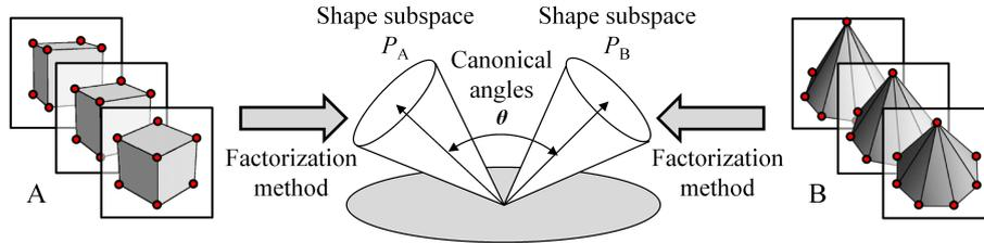
**Fig. 1.** Proposed framework of 3D object recognition based on canonical angles between shape subspaces.
