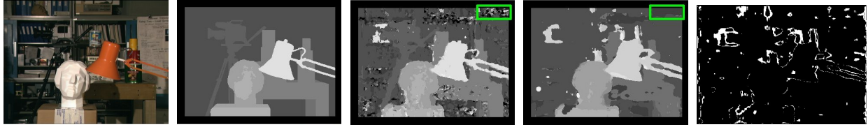
Figure 5: From left to right: Left image from the original head and lamp dataset, ground-truth disparity, disparity map with cost-minimization method, disparity map with learning-based approach, and the confidence map.
