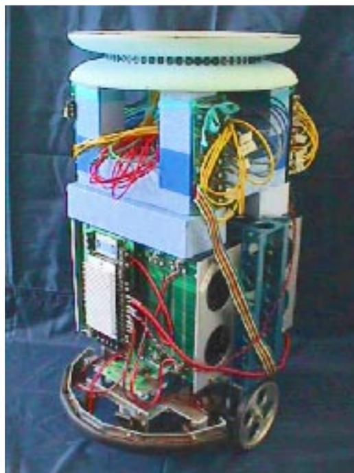
Fig.1: A mobile robot “Yamabico AO” with a sonar ring sensor – ONSiDe.
