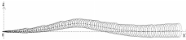
Figure 10: Estimated position and error variance with correction. The error variance of z is corrected, and is kept small. The correction is executed every 4 seconds. (Notes: the magnification of z coordinate is around 1.5 times as long as x coordinate.)
