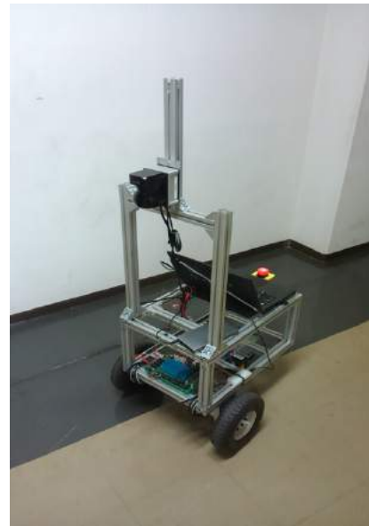
Fig. 4 Wheeled Robot used for Map Building
