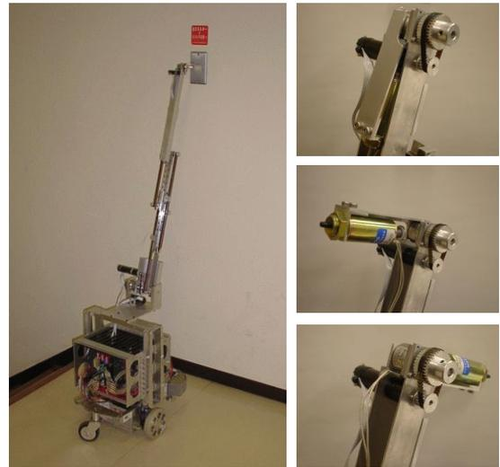
Fig.9 Expanded arm and End-effector
