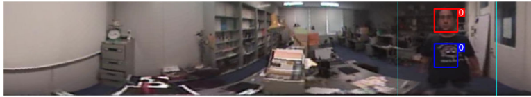
Fig. 6. Result of the face detection algorithm (red) and the position of the patch extraction (blue), the number is the index of the detected face
