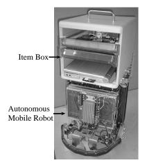
Figure 2: Autonomous mobile robot "Yamabico" supporting the item box
