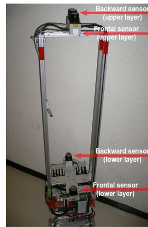
Fig. 3: Our robot system for multiple people detection and tracking, four URG-04LX are used.
