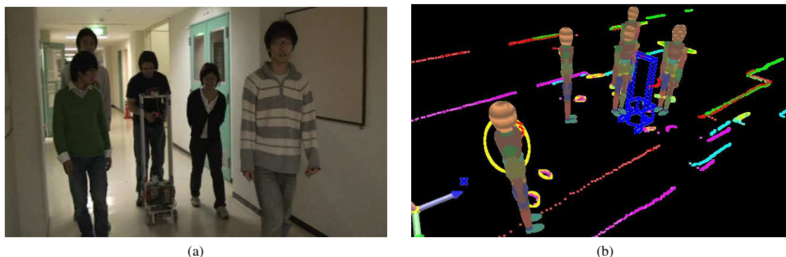
Fig. 8: Results of the people detection, (a) snapshot (b) 3D models in estimated positions of people in the experiment.
