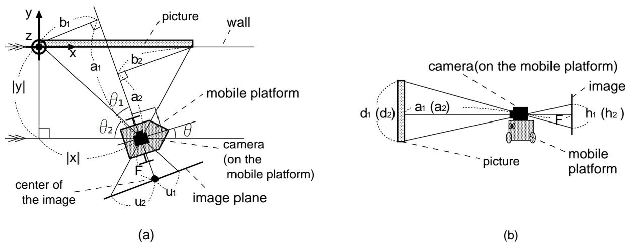
**Fig.2** Method of calculating the positional relationship of the picture, the robot and camera ((a): Overhead view, (b): Side view)
