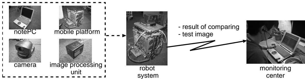
**Fig.9** Structure of the robot system
