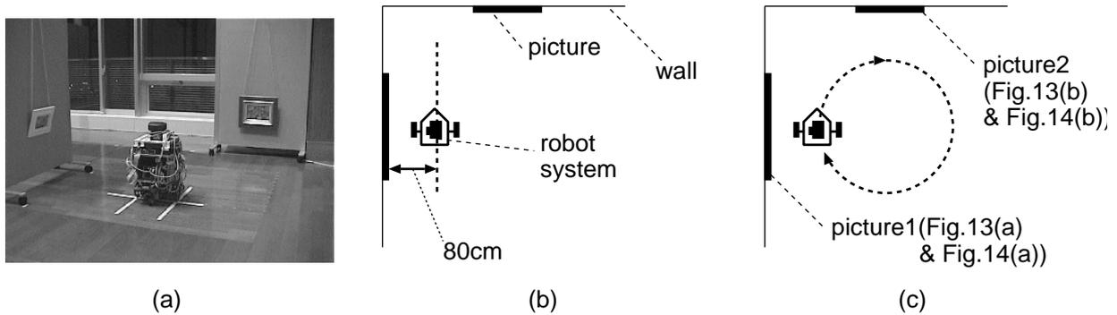
**Fig.12** Actual experiment of the monitoring system ((a): A view of the experiment, (b): Overhead view of the environment in the experiment, (c): Patrolling route and target pictures for monitoring)
