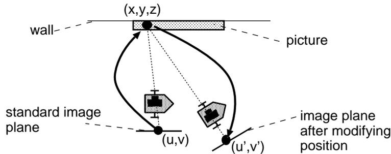
Fig.4 Positional relationship of the robot and a picture used for modifying the image
