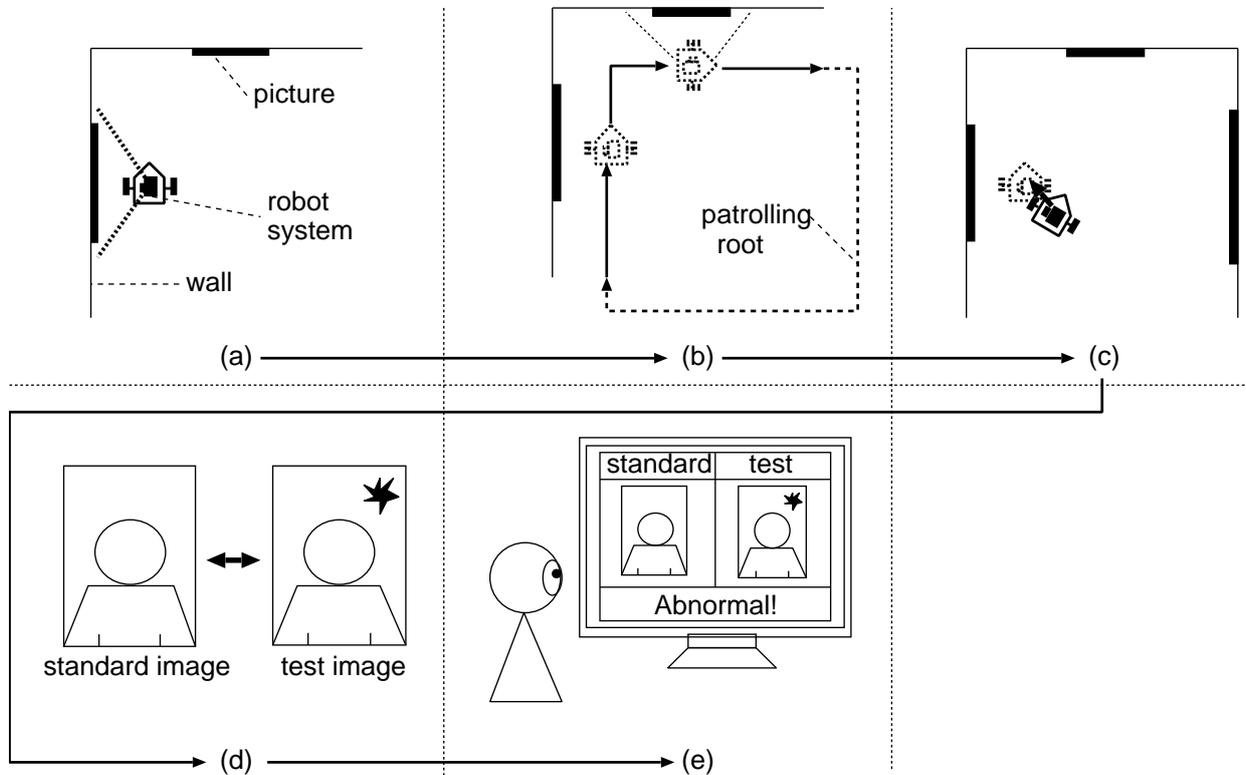
**Fig.10** Action of the monitoring system ((a): Taking a standard image and calculating the robot's position, (b): Taking standard images and calculating a robot's positions for all pictures, (c): Taking an image after moving and correcting a robot's position, (d): Taking a test image for modification and comparison with the standard image, (e): Sending a comparison result)
