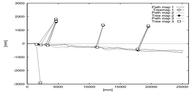
Figure 12: The generated route maps: Path map 1 and Tree map 1 indicate the routemap in the first trial. The points of Tree map indicate the pair of the sensing point and the landmark location.
