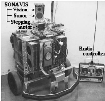
Figure 6: The YAMABICO NAVI robot for the teaching playback navigation robot system(to change the current robot)
