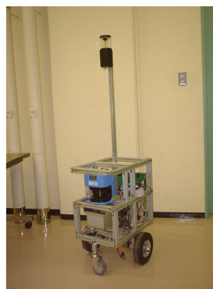
Figure 1: The mobile robot equipped with an omnidirectional vision sensor and a laser range finder.
