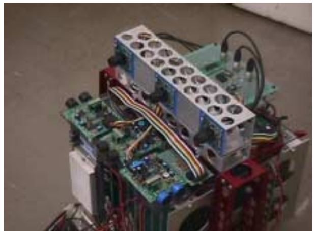
Fig. 8. The trinocular vision sensor mounted on the robot.
