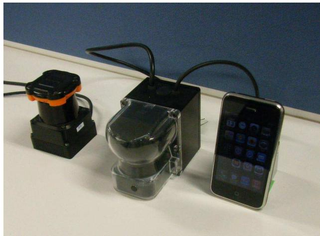
Fig. 9. Second prototype sensor, which is at the center. UTM-30-LX sensor and a smart phone (iPhone3) are placed on the left and right to compare their sizes.
