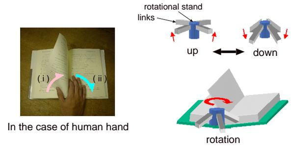
**Figure 4:** Structure of page turning device.
