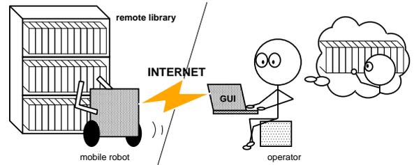
**Figure 1:** Concept of remote book browsing system using a mobile robot.
