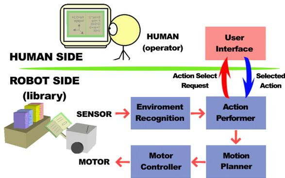
Figure 5: Control system of teleoperation.
