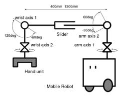
Fig. 3. Hardware Diagram of the Manipulator
