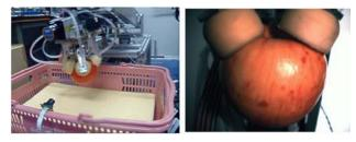
Fig. 9. Camera Attached to the Basket (left), and An Image Captured by the Basket-Camera (right)
