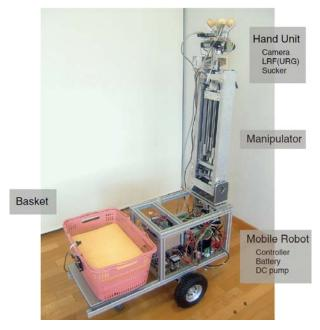
Fig. 5. The Integrated Shopping Robot
