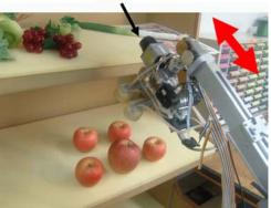
Fig. 6. Small LRF (URG) Attached to the Robot Hand.
