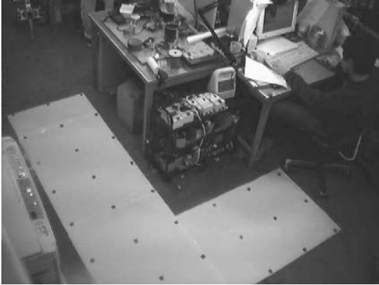
Fig. 6 Grid sheet used for finding coordinate transformation parameters by least square method
