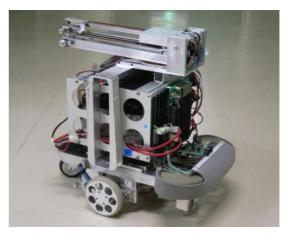
Figure 7: Contracted arm on mobile robot.
