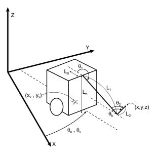
Figure 8: Mobile arm coordinate system.
