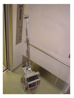
Figure 10: Pushing an elevator button.
