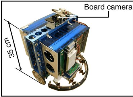
Figure 7: The YAMABICO robot with its top board camera.
