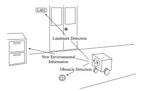
Figure 2: Sensing needed on navigation.
