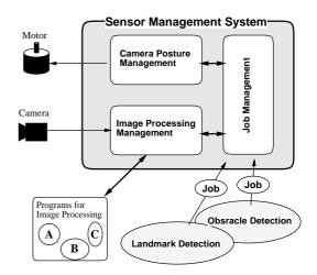
Figure 3: Structure of sensor management system.
