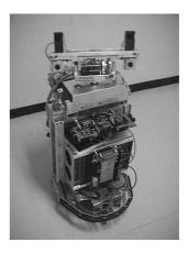
Figure 1: Autonomous Mobile Robot "Yamabico" equipped with the active stereo vision sensor system.
