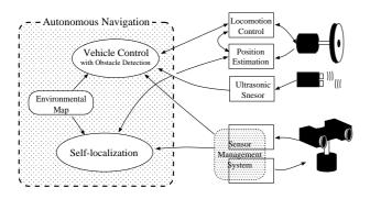
Figure 5: Structure of navigation software.
