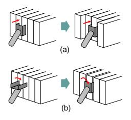
*Figure 4: Method for book grasping. (a) A vertical modality push the book into an undesirable situation. (b) Entering an inclined trajectory.*
