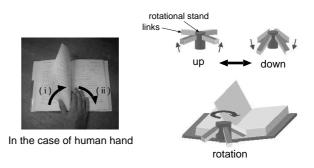
Figure 9: Structure of page turning device.
