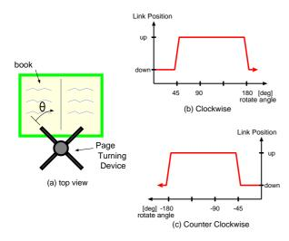
*Figure 10: Timing chart of page turning device. (a) model, (b) turning on the right, (c) turning on the left*
