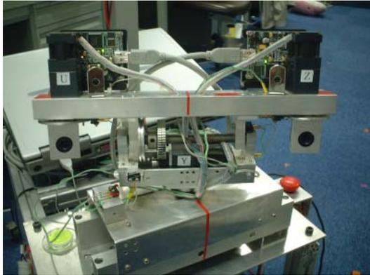
Fig. 6. Stereo camera mounted on the Pan-Tilt device.
