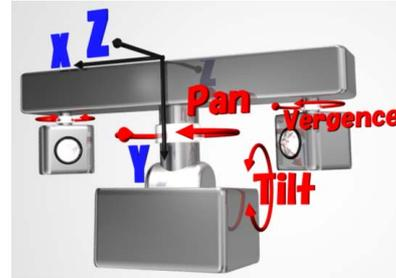
Fig. 10. Definition of a coordinate system.
