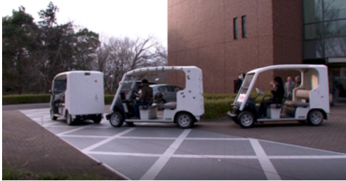
Fig. 2. Traveling experiment with golf carts as prototype vehicles.
