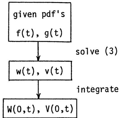
Figure 1 Conventional approach for computing  $W(0,t)$  and  $V(0,t)$
