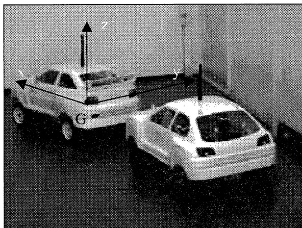
Figure 2 : definition of vehicle's axis
